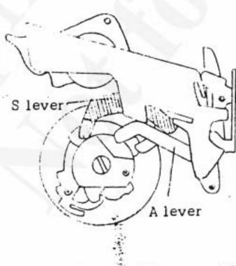
Action is transmitted from 8606 to the S lever and from 8605 to the A lever, while both the L ankle and the S ankle remain off the engagement. Without the use of the Ankle, the load is given only by the gears. Differentiation between 1/15 and 1/30 will be in the same manner as in the case of 1/1 - 1/8.
