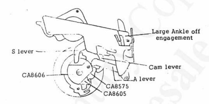
The S lever escapes from 8606 and the S ankle is engaged. 8605 pushes the A lever and the L ankle remains unengaged. To differentiate the shutter speeds of 1/4 and 1/8 from each other, the message is transmitted from 8575 to the Cam lever to change the operating angle of the G lever.
