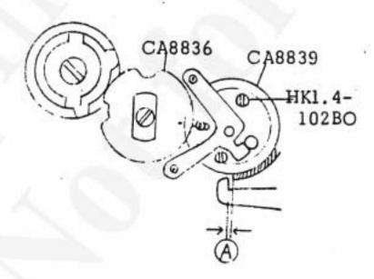
Prior to film advancement, when the Gear A is pressed in the arrowed direction, the distance between 8840 and the Gear A should be  $-0.10 \sim +0.3$ . (-0.10 means the state where the Gear A comes in contact with 8840 and further moves by 0.1.)
