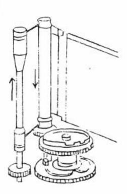
1st curtain stops at the improper position.
