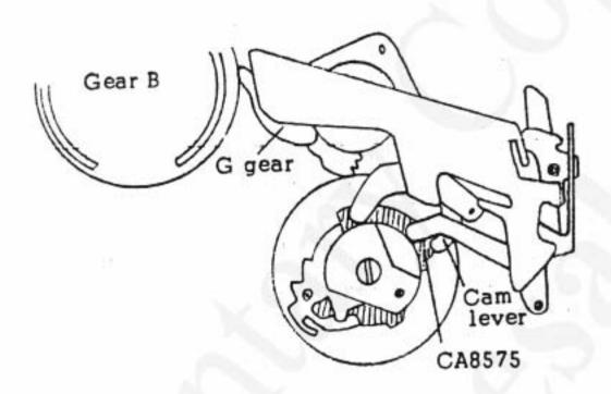
In cases of 1/60 - 1/1000, the action is transmitted from 8575 to the Cam lever of the Governor then to the G gear, and the arrowed portion of the Gear B is disengaged from the G gear. The governor will not be activated in this case.
