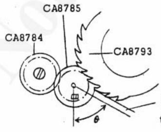
The clearance between boss of 8785 and 8793 should be over than lmm.
