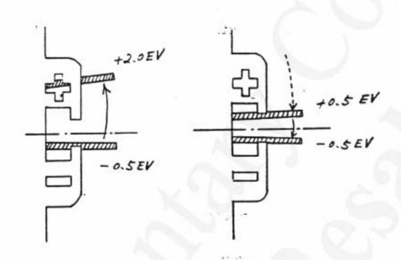
When the lens aperture is stepped down from the wide open state, the meter needle should once swing down to a position lower than -0.5EV before it is stabilized at +0.5EV. (See Fig. B.)
