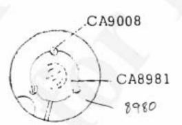
Fine adjustments are made by 9016 (a part of 8995 assembly). At this time, it is preferable not to loosen 9016.
