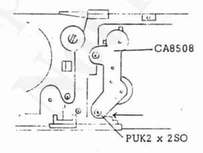
In case where the Shaft rattles vertically due to deformation of 8508, insert a U washer (0.1 - 0.2) underneath the Plate R on the arrowed side.
