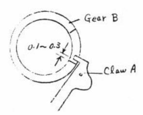
When Claw A is shaken if its lower edge hits the Gear B, an adjustment may be made by bending the Plate (B).
