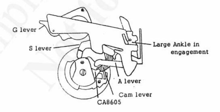
The A lever is released from 8605 and the L ankle is engaged. The S ankle remains off engagement by the S lever. To differentiate shutter timing for 1/1 and 1/2, the message is transmitted from 8575 to the Cam lever and the operating angle of the G lever will be changed.
