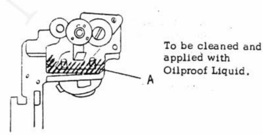
(4) Before mounting the Top cover, check the operation of CA8995. Upon mounting the Top cover, check the indicator accuracy. Ref: E-39
