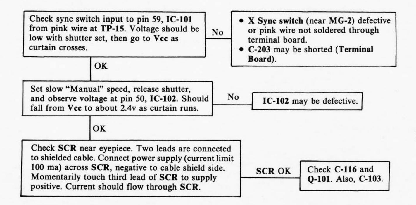
Note: With top off, shield side of cable to SCR must be grounded to strap lug for flash socket to work. Also, mirror safety switch connects flash socket to SCR through center lead of shielded cable.
