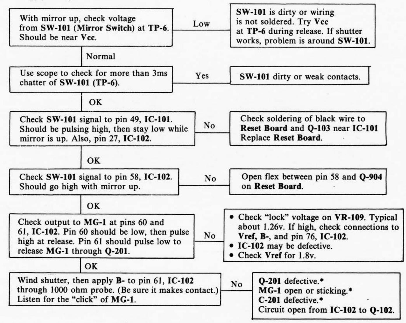
\* Q-201, C-201, and MG-1 are on the board under the mirror. They can be reached by removing the cover plate in front.
