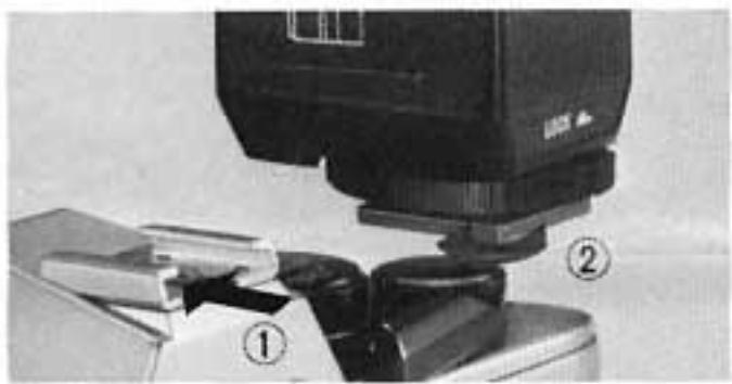
Slide the extender into the accessory shoe and tighten the lock knob.
