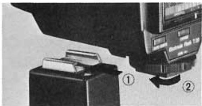
Slide the flash unit into the extender (top) and tighten the lock knob.
