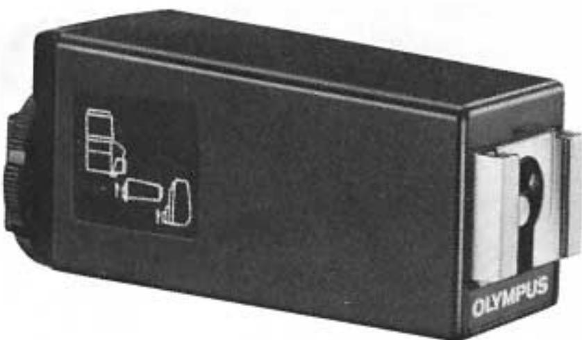
The flash extender widens the distance between the flash surface and camera lens to virtually eliminate the possibility of 'red eye' effect in on-camera direct flash photography.
