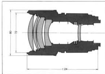
Notwithstanding its 180mm focal length, this lens features a fast F2.8 speed, making it an ideal telephoto for dim light photography. Generally in indoor sports arenas and theatres, the use of flash light is prohibited, rendering slow shutter speeds inevitable and imposing a difficult task upon the photographer. This unusually bright telephoto, however, permits higher shutter speeds and, being small and light, makes focusing quick and easy enough to catch fast action even in dim-lit situations.
