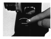
To lock the Shutter Release of the Control Grip, turn the Shutter Release Lock Lever in the direction of the arrow until it stops with a click.
