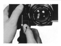
③ To remove the Control Grip, push in and down on the Grip Detach Button to disengage the Grip Locks, and then lift apart.
