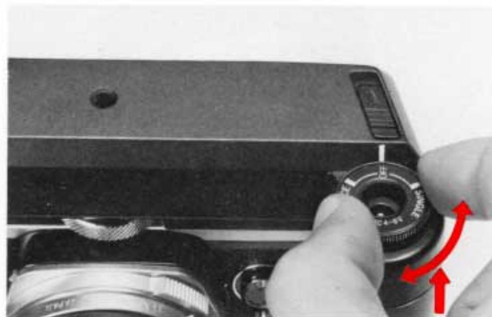
Turn the Fastening Screw clockwise until the Winder 2 is securely attached to the camera base plate. To detach, turn the Screw counterclockwise.
