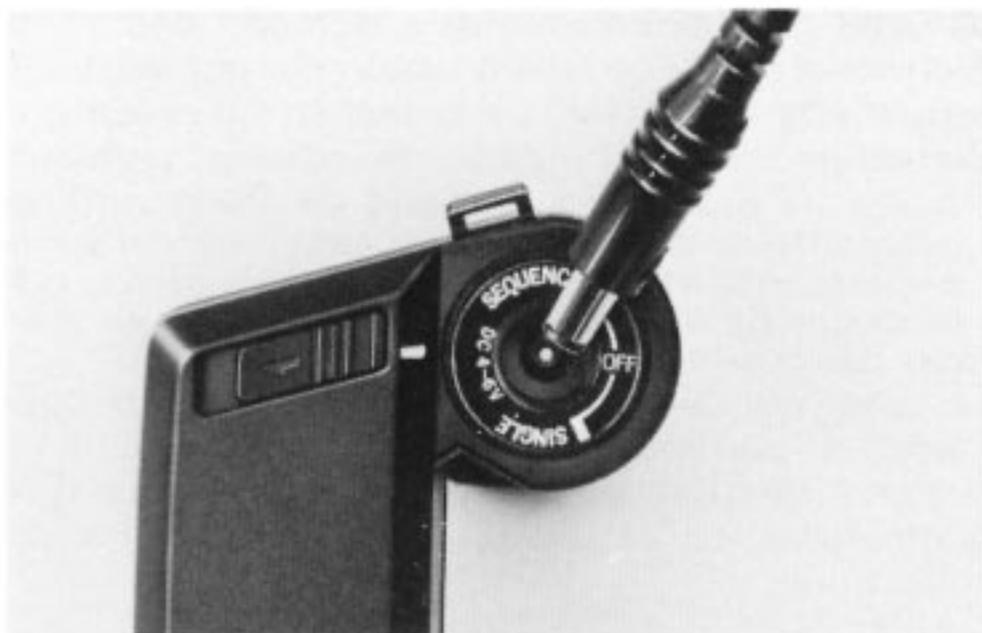
1. The External Power Jack at the center of the Mode Selector accepts the power plug from an external power unit of up to DC 6V (4–5.5V with a power unit of large potentiality).
