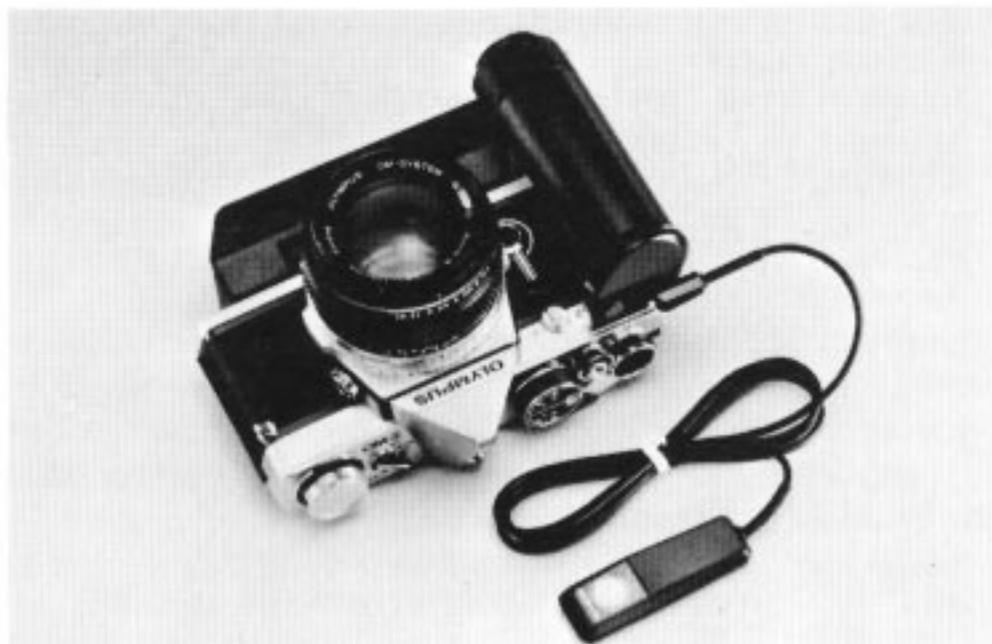
The Remote Control Jack provides a facility for remote motor drive photography. The jack accepts a 2.5mm mini-plug (output terminal of remote control apparatus). There are two optional M. Remote Cords available from Olympus in 1.2m and 5m lengths.
